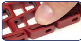
After rod is positioned, place plug and push it into position with your thumb.
