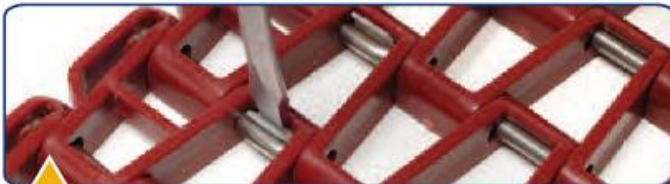
Insert a flathead screwdriver between the flag and the belt. Strike screwdriver with hammer to dislodge the flag.
