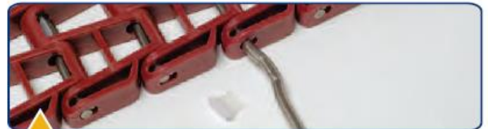
After the flag is removed, the rod can be pushed out with a punch or screwdriver.
