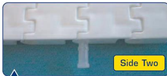
The head will be exposed on the other side of the belt.
