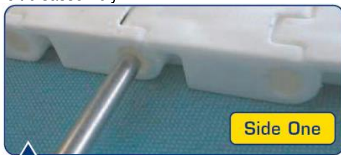
Put a nail punch on the unheaded side of the rod and hit with a hammer.
