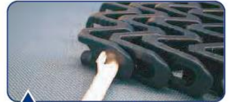
▲ Rotate pins approx. 45° and slide pin into the belt (one from each side and thick end first).
