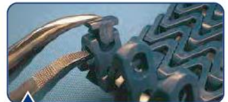
▲ Use nose pliers to put plug into final position.
