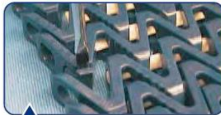
▲ Use flat blade screwdriver to pry out the plug.
