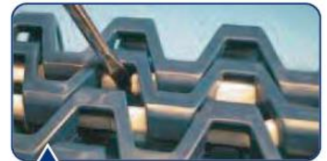
▲ Use flat blade screwdriver to pry out the rods.
