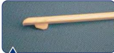
▲ Tapered pins. There are two pins per row.
