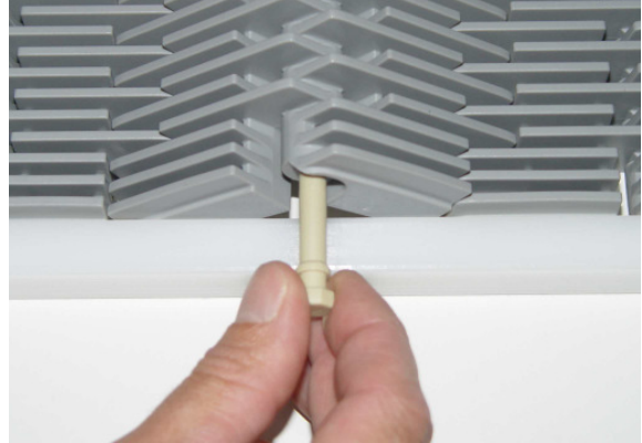
Insert rod For easy installation rod end must be beveled.
