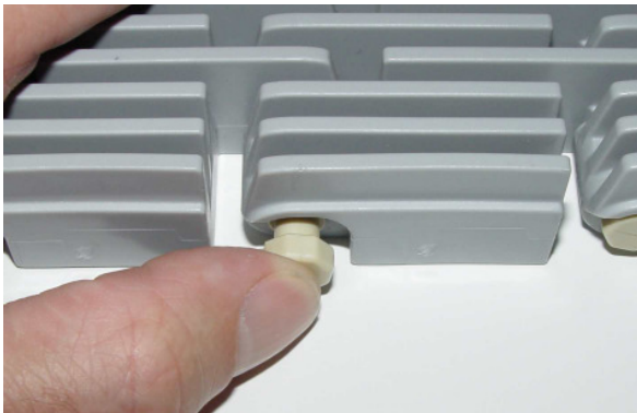
Push-in rod head Check if rod head is fully embedded.
