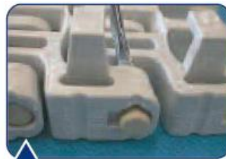
Use a flat screwdriver to push the head partly out of the finger until the head is exposed.
