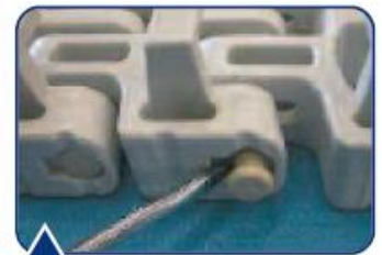
Use a screwdriver to pull out the head of the rod completely. After this, use a pin to push out the remaining rod.
