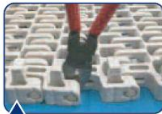
Use a gate cutter to cut the end rod on both sides of the retainer ring. (First cut "inner" side, then cut the "outer" side.)
