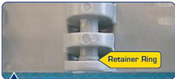
Use a gate cutter to cut the end rod on both sides of the retainer ring, just inside of the first finger. (First cut the "inner side", then cut the "outer finger" side).
