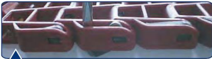
Push the plug down with a screwdriver until it comes out of the module.
