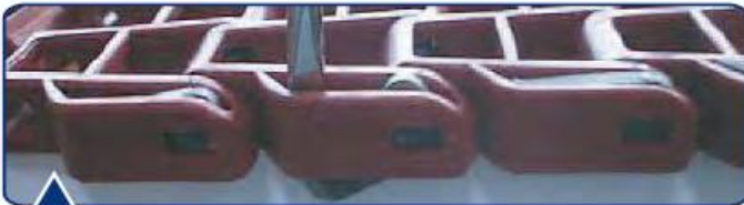
Push the plug down with a screwdriver until it comes out of the module.
