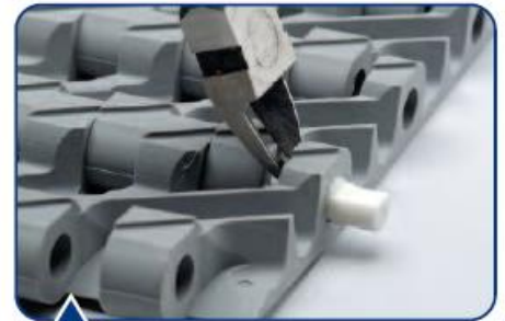
Use cutters to push out rodlets from each side and then remove floater.
