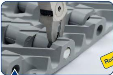
Cut "snap" off the rodlet (repeat process on other side of belt).
